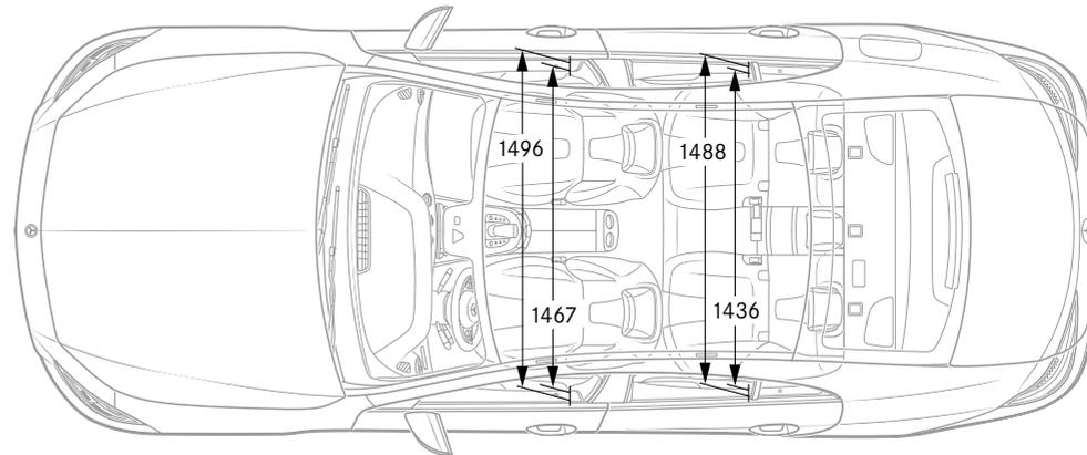
All figures in millimetres. The dimensions shown are median values. They are applicable for unladen vehicles in the standard specification.
